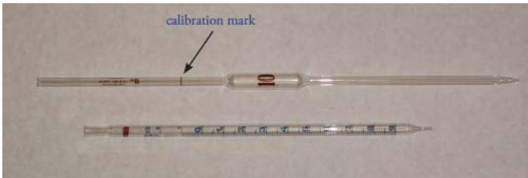
**Figure 2.5** Two examples of 10-mL volumetric pipets. The pipet on the top is a transfer pipet and the pipet on the bottom is a Mohr measuring pipet. The transfer pipet delivers a single volume of 10.00 mL when filled to its calibration mark. The Mohr pipet has a mark every 0.1 mL, allowing for the delivery of variable volumes. It also has additional graduations at 11 mL, 12 mL, and 12.5 mL.
