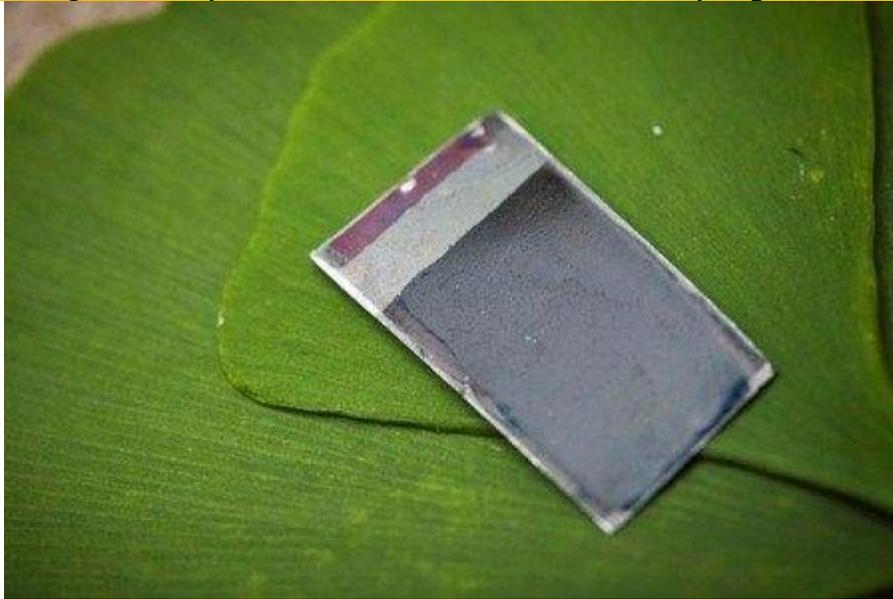
This Leaf device combines a commercially available solar cell (Silicon) with a pair of inexpensive catalysts made of Cobalt and Nickel that split water into Oxygen and Hydrogen. The hydrogen can be stored and used as an energy source. (For example to power a fuel cell).
