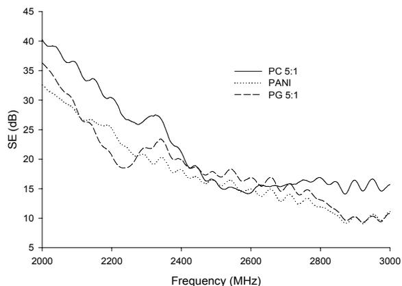
Fig 4. Shielding efficiency for different composites
