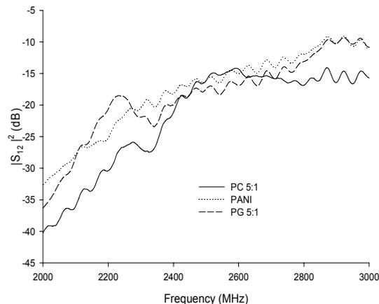
Fig.3 Variation of Transmission coefficient for thickness 7.5 mm
