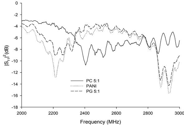
Fig 2. Variation of Reflection coefficient for 5mm thickness
