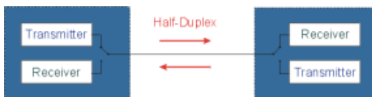
Figure 2 - Half Duplex Communications
