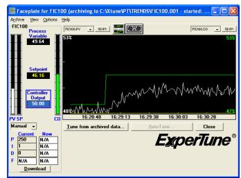
model, accept the proposed tuning, and simulate the results directly from their desktop. After communicating the change to operations, the new tuning can also be downloaded directly from the desktop.
