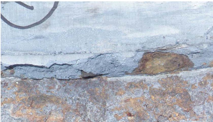
**Figure 2\*. Pipe sample showing corroded steel and cement surface below X-Pando sealant**
