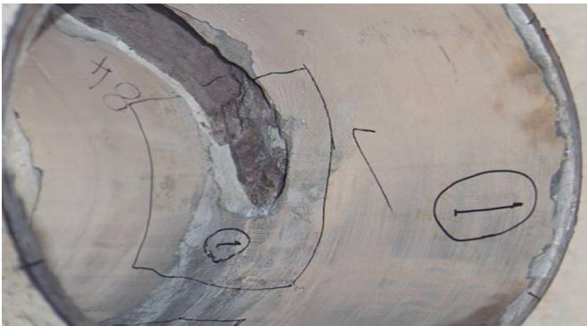
**Figure 1\*. Disbondment of X-Pando sealant**
