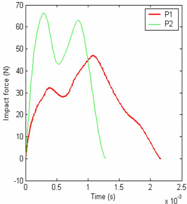
Fig. 7. Impact force of sandwich plate P1 and P2 for an initial impact velocity  $V_0 = 1\text{m/s}$ .
