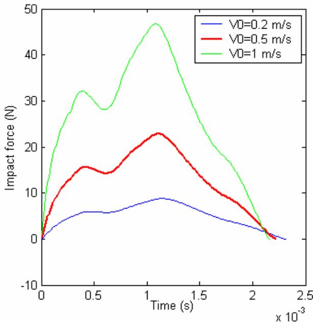
Fig. 3. impact force on the sandwich plate P1
