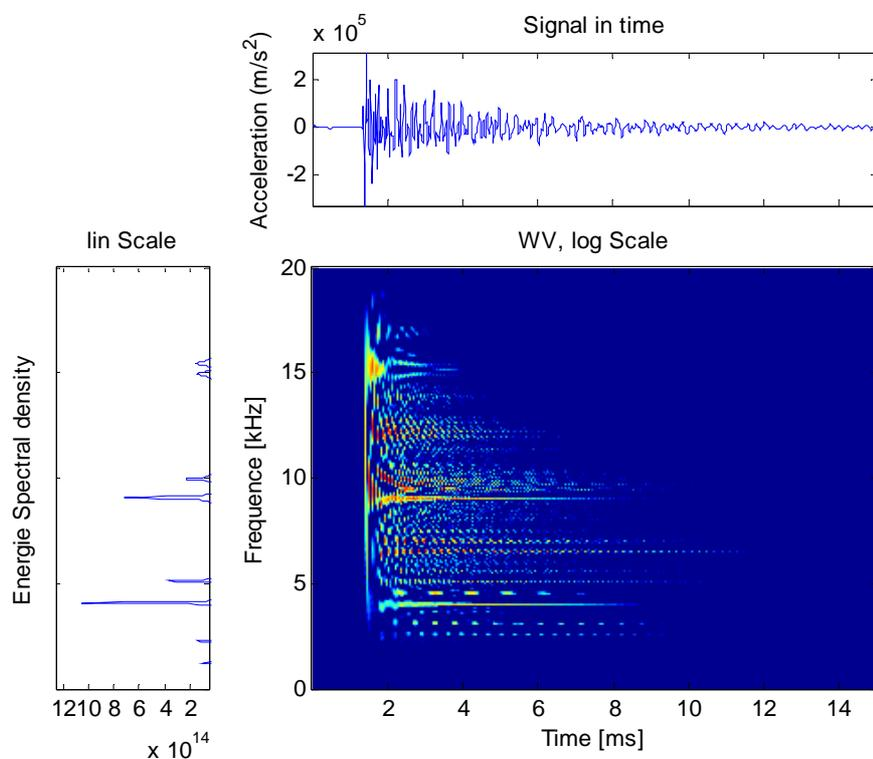
Fig. 11. Wigner-Ville Distribution, frequency response and temporal response of the Sandwich plate P2 under impact of a sphere with an initial velocity  $V_0=1m/s$ .
