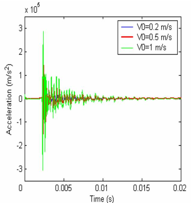
Fig. 6. Temporal responses of impacted sandwich plate for different initial velocity of impactor.
