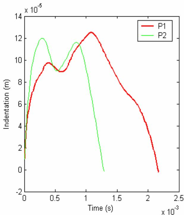
Fig. 8. Indentation of sandwich plate P1 and P2 for an initial impact velocity  $V_0 = 1\text{m/s}$ .
