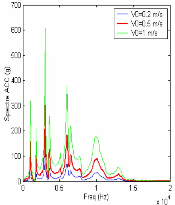
Fig. 5. Frequency responses of impacted sandwich plate for different initial velocity of impactor.
