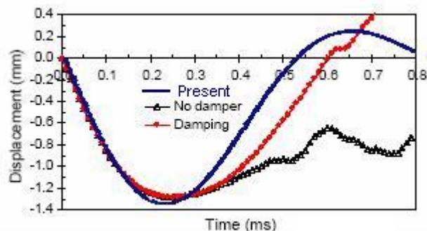
Fig. 2. Comparison of displacement history for a steel plate.
