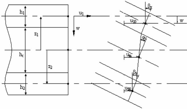
Fig. 1. Sandwich plate displacements in the x-z-plane.
