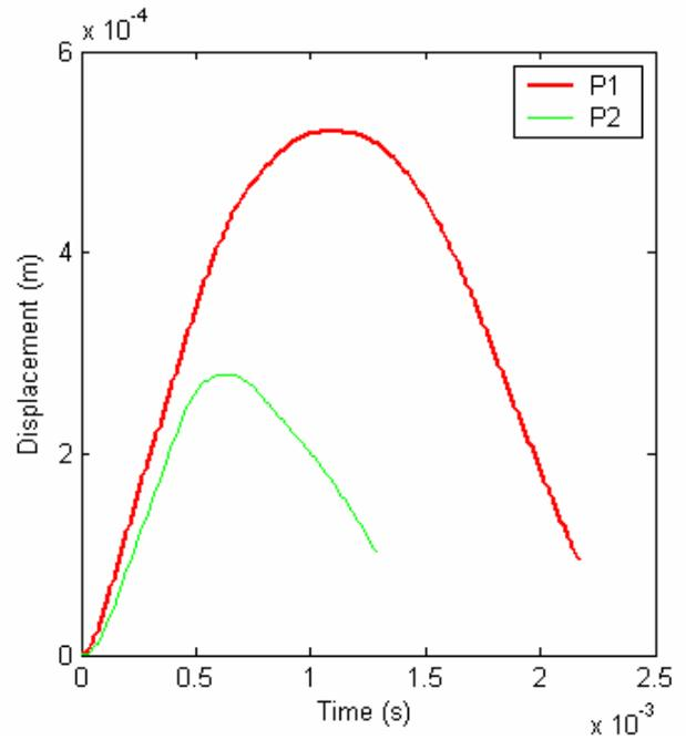
Fig. 9. Displacements of the center plates for an initial impact velocity  $V_0 = 1\text{m/s}$ .
