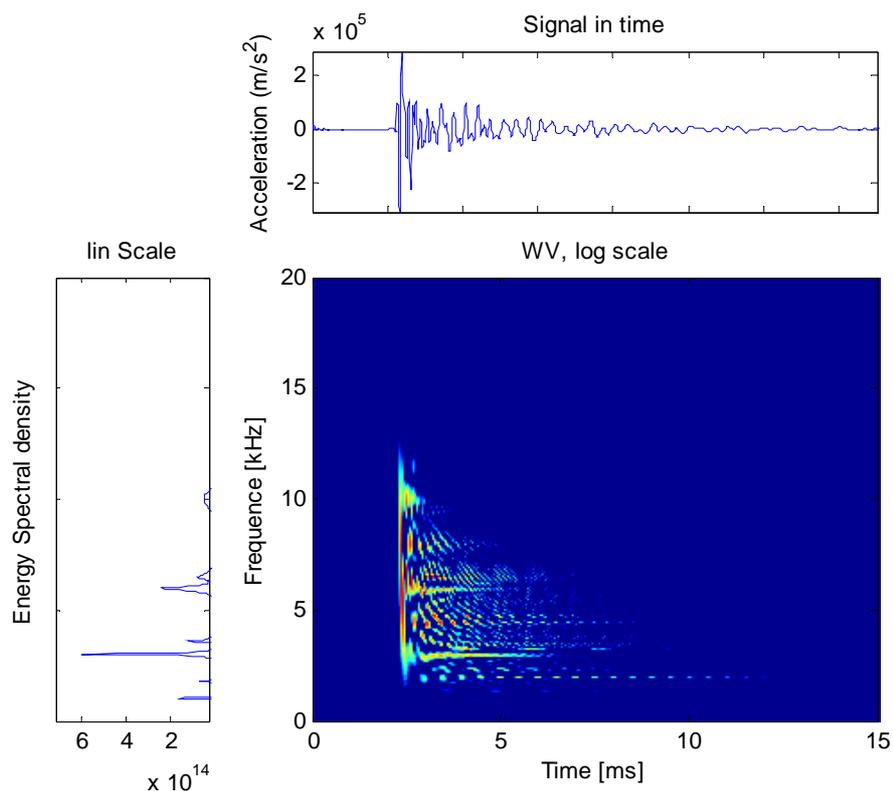
Fig. 10. Wigner-Ville Distribution, frequency response and temporal response of the Sandwich plate P1 under impact of a sphere with an initial velocity  $V_0=1m/s$ .
