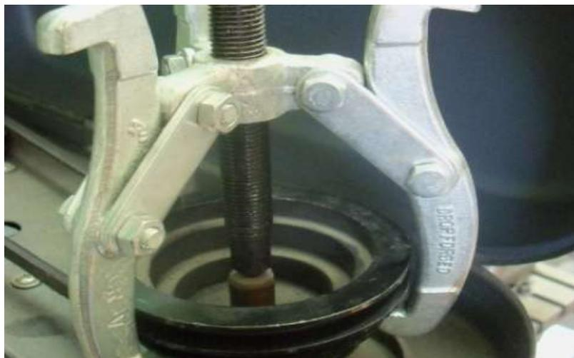
Once you have determined how a pulley is fitted to the motor and you are sure you have unscrewed any grub screws etc, the easiest way to remove it is with a gear puller. The pulley is ‘jacked’ off of the motor shaft by turning the central bolt of the gear puller using a spanner. The image above is for illustrative purposes, as you must remove the drive belt and isolate the machine from the electric supply first.
