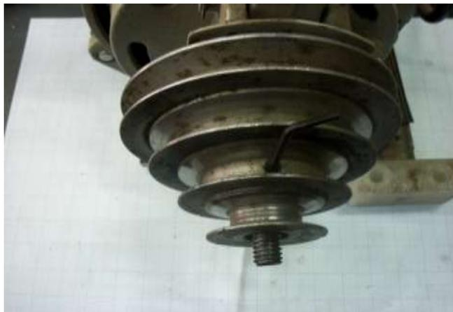
Above you can see how the pulley can now be fixed to the sleeve by using a grub screw into the 'D' dent.
