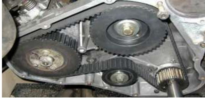
As well as these 'vee' or 'wedge' type pulleys, you may come across pulleys which appear to look like gears. These are normally found in engines not on electric motors. It can be very costly to buy belts or matching pulleys if you intend to use them. Also shown in the image above is an 'tension pulley'. This is the small pulley in the centre. It will have some way of moving up and down and used to tension the drive belt. You can buy standard tension pulleys sets off of the internet.
