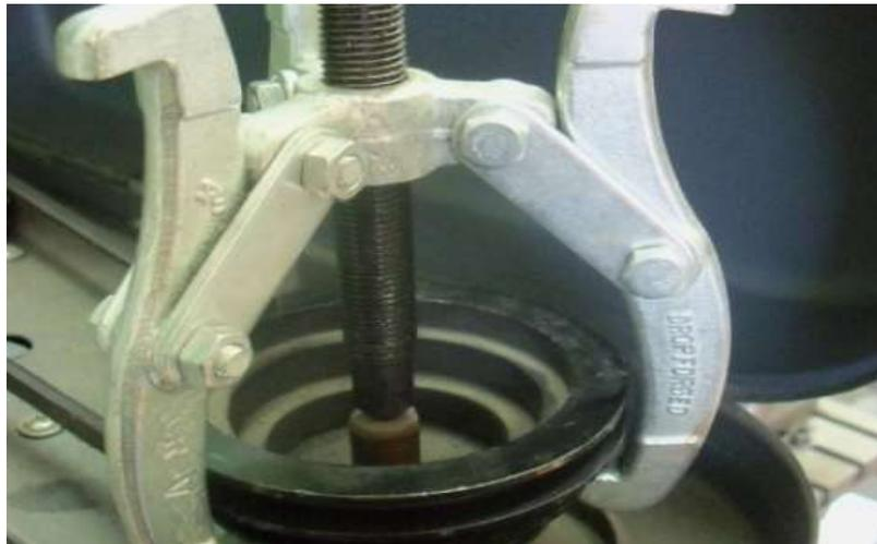
Once you have determined how a pulley is fitted to the motor and you are sure you have unscrewed any grub screws etc, the easiest way to remove it is with a gear puller. The pulley is ‘jacked’ off of the motor shaft by turning the central bolt of the gear puller using a spanner. The image above is for illustrative purposes, as you must remove the drive belt and isolate the machine from the electric supply first.
