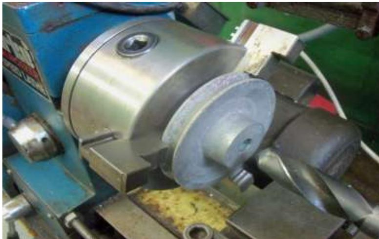
I recommend using the 'outside' jaws to grip the pulley unless there is a nice long parallel section to hold in the chuck.
