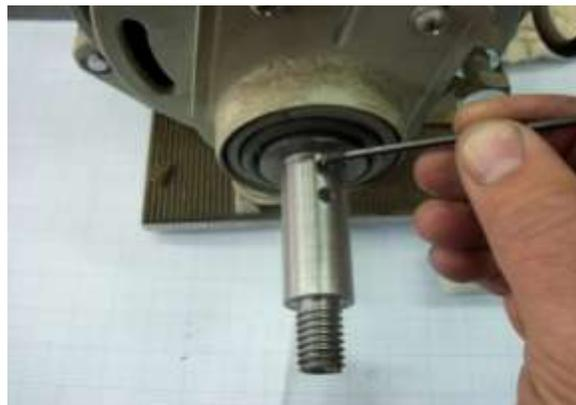
The sleeve is fitted securely to the motor shaft with 2 grub screws that line up with the keyway.
