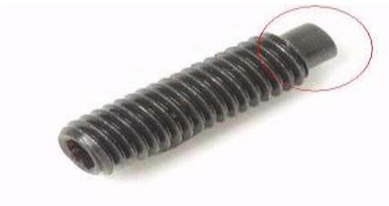
These are small screws that are tightened with a ‘hex key’ better known as an ‘allen key’. It’s important to make sure that the grub screw is fastened into the keyway of the motor shaft and not onto the shaft itself, otherwise the pulley will come loose and the motor shaft will get damaged.
