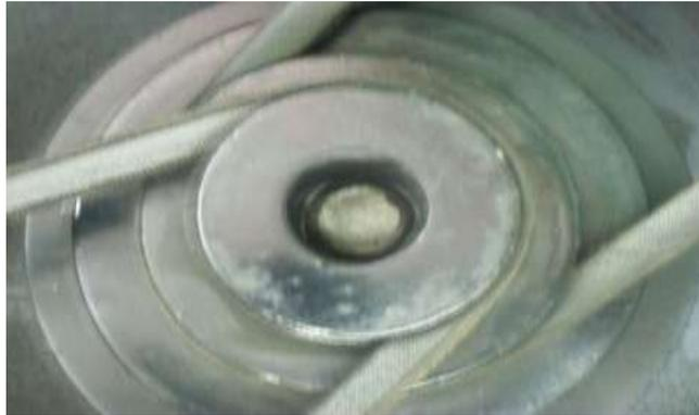
Better known as 'idler wheels' are used to alter the rpm of the final drive. By placing an idler wheel in between the motor pulley and final drive we can reduce or increase the drive speed. Idler wheels are not powered in themselves, they simply transfer drive via the vee belt. The spindle for the idler wheel will need to run freely in bearings.
