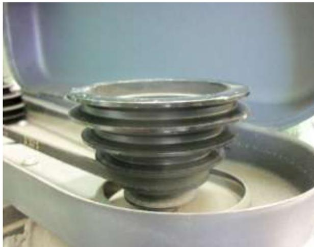
Pulleys are commonly used if the motor is going to rotate at high speed, but not always as I have seen them used in heavy duty mirror ball motors. The drive is transferred to another pulley using a vee belt (both pulley and vee belt are shown in the image above).
