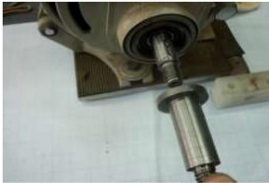
Once machined the sleeve is slid over original motor shaft.
