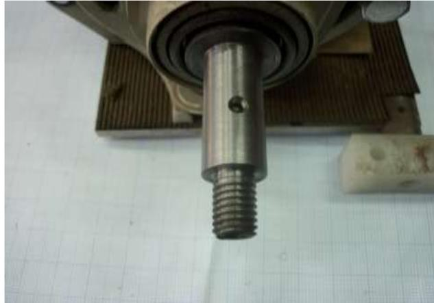
In the image above, the sleeve has been secured to the motor shaft with two grub screws, the motor shaft (with the sleeve secured) has been rotated to show a 'D' dent which has been machined into the other side.
