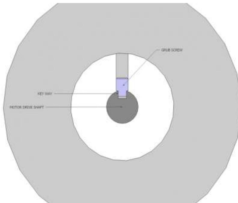
If there is nowhere obvious on the pulley to drill and tap a grub screw, you can drill into the bottom of one of the grooves as shown below, however, you must ensure you have removed any sharp edges afterwards and that the grub screw is well below the surface so as not to interfere with the vee belt.
