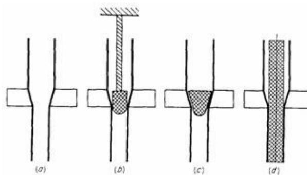
Fig. 6: Tube drawing processes
