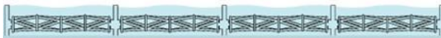
Multiple THAWT rotors can be chained together across the width of channel
