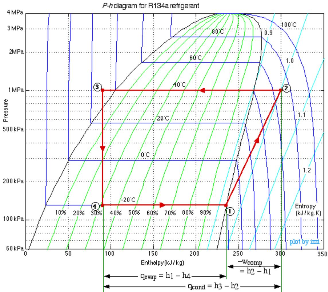
Notice from the *P-h* diagram plot how we can get an instant visual appreciation of the system performance, in particular the Coefficient of Performance of the system by comparing the enthalpy difference of the compressor (1)-(2) to that of the evaporator (4)-(1) in the case of a refrigerator, or to that of the condenser (2)-(3) in the case of a heat pump.
