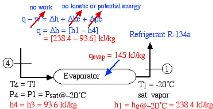
In determining the Coefficient of Performance - for a refrigerator or air-conditioner the desired output is the evaporator heat absorbed, and for a heat pump the desired output is the heat rejected by the condenser which is used to heat the home. The required input in both cases is the work done on the compressor (ie the electricity bill). Thus
