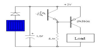
This design can be used for BEAMbots that you only want to be active at night -"crickets", night-lights, and such "pummers." Note that you could just as easily
