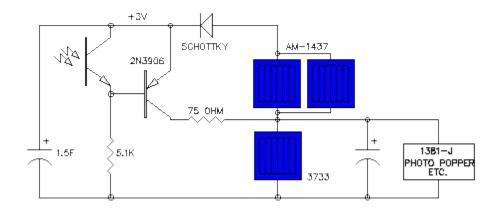
In this diagram, the "SmartCap" is just the 1.5 F storage capacitor, phototransistor, 2N3906 transistor, and 5.1K bias resistor. The idea is that after charging, a loss of light causes the 1.5 F capacitor to be discharged through the 75 Ohm resistor -- this gives the photopopper a sudden "recharge," which it can use to get to a brighter spot.
