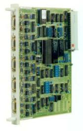
Fig. 22.6 A high speed counter module
