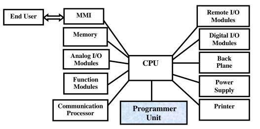
Fig. 22.1 Typical Subsystems for a PLC system
