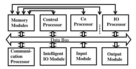
Fig. 22.2 Functional hardware organization of a PLC System
