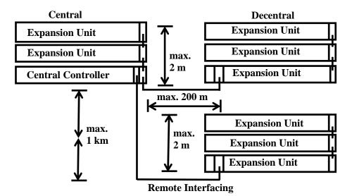
Fig. 22.3 Physical layout and Bus extension System for PLCs
