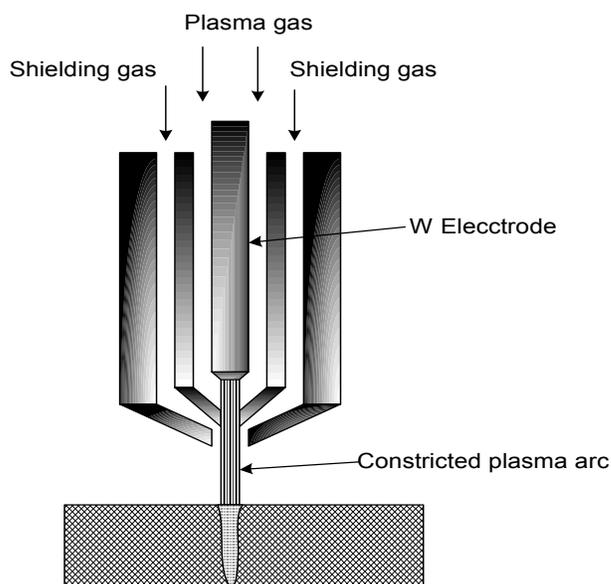
Fig. 16.6 Schematic of constriction of arc in PAW
