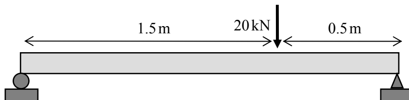
Figure 7.4.27: a simply supported beam
