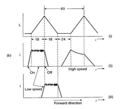
Applying the stator pulse when the inductance profile has positive slope induces forward motoring torque.
