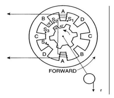
The stator poles have concentrated winding rather than sinusoidal winding. Each stator-pole pair winding is excited by a converter phase, until the corresponding rotor pole-pair is aligned and is then deenergized. The stator-pole pairs are sequentially excited using a rotor position encoder for timing.
