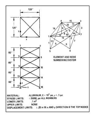
Fig. 4 : Nodal Position and Material Properties of 72 Truss Example
