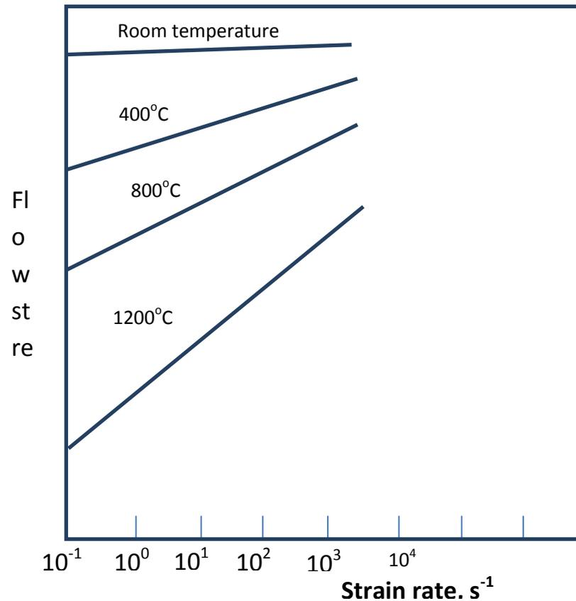
**Fir. 3.3.4.1.1: Variation of flow stress with temperature and strain rate**
