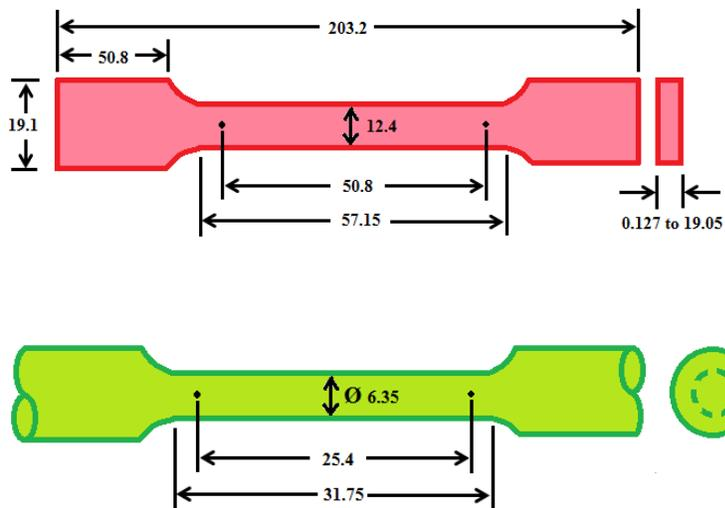
**Fig. 3.3.1.3: Standard (ASTM E8) Tensile Specimens of plate and cylindrical types**
