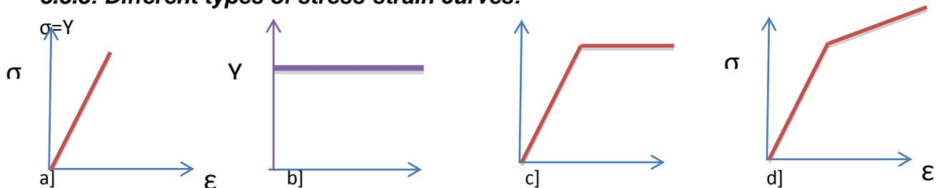
**Fig. 3.3.3.1: Stress-strain behavior of different types of materials**
