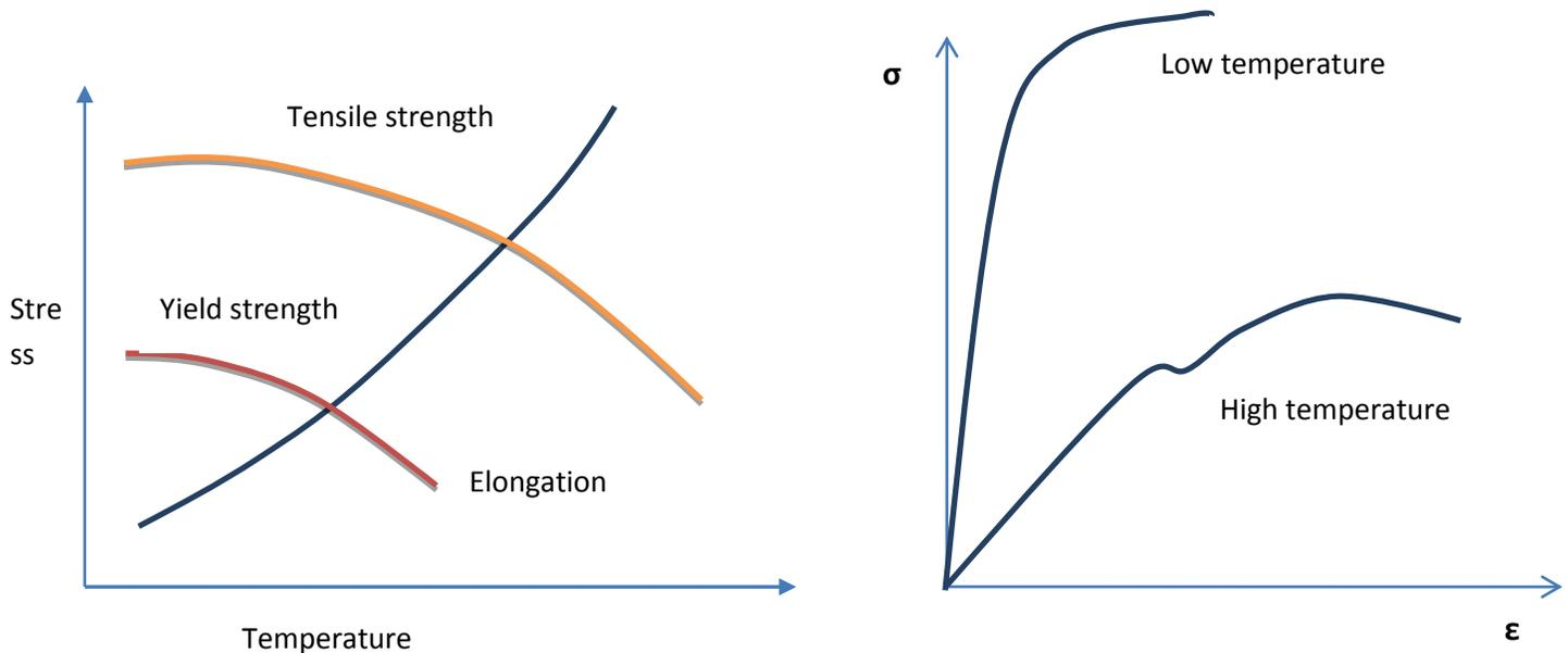
**Fig. 3.3.4.1: Effect of temperature on mechanical properties and stress-strain behaviour**
