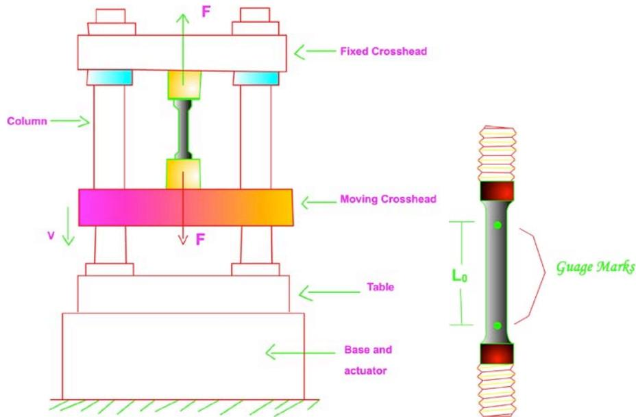
**Fig. 3.3.1.2: Tensile test setup and tensile specimen**
