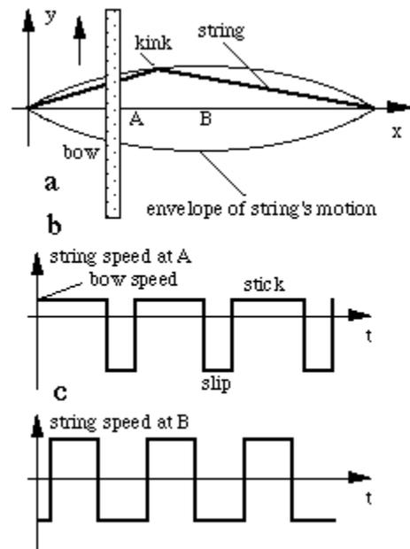
there is a large transient force on the string (the tension on both sides of the string now has downwards components). This starts the slip phase ( $v < 0$  in figure b) during which the kink travels to the left hand end, is reflected and returns to the bow, ready to being the stick phase again. At the midpoint of the string (B), the up and down speeds are equal (figure c).
