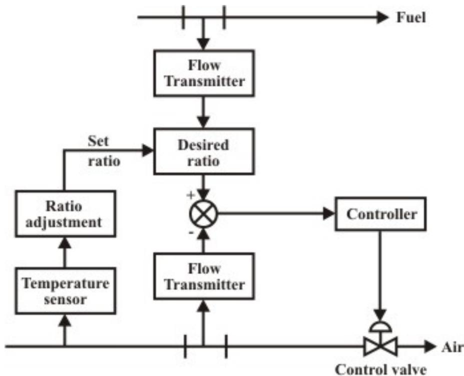
Fig. 7 Ratio control with ratio adjustment mechanism
