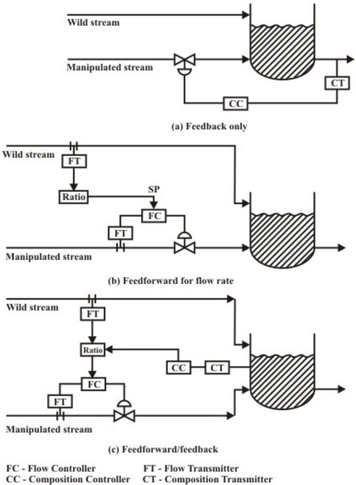
**Fig. 8 Comparison among Feedback, Feedforward and Feedforward-feedback Control**
