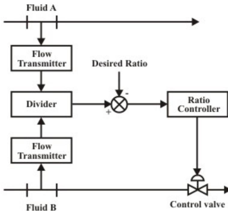
Fig. 5 A possible configuration for achieving ratio control
