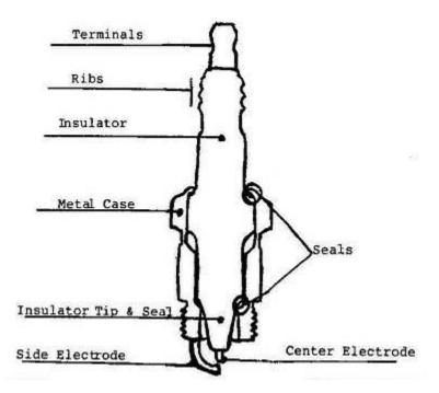
A spark plug is composed of a shell, insulator and the conductor. It pierces the wall of the combustion chamber and therefore must also seal the combustion chamber against high pressures and temperatures, without deteriorating over long periods of time and extended use.
