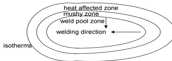
Fig. 33.5 Schematic showing different zones
