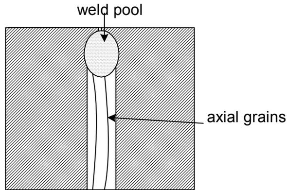
Fig. 33.9 Schematic of axial grain in weld joints
