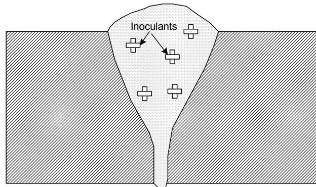
Fig. 33.11 Schematic of grain refinement by inoculation
