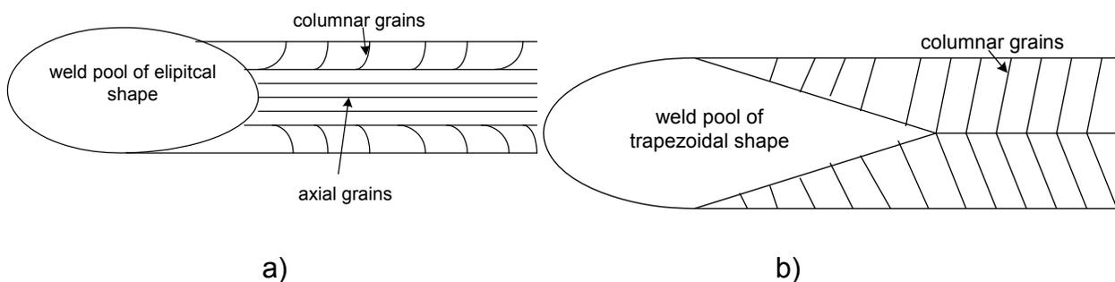
Fig. 33.10 Effect of welding speed on shape of weld pool and grain structure at a) low speed and b) high speed
