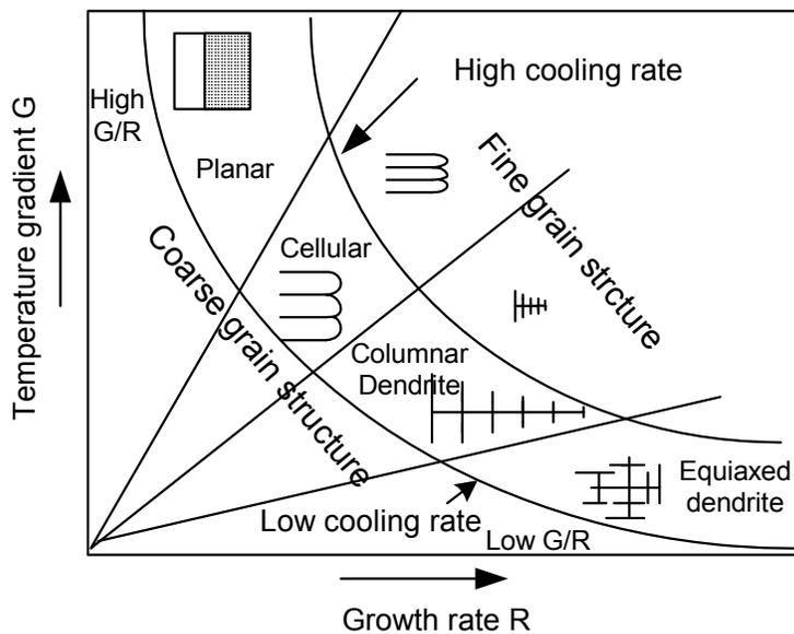
Fig. 33.4 Influence of  $G$  &  $R$  on mode of solidification and grain structure
