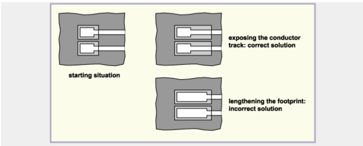
Footprints for MELFs and chips should extend far enough to provide an aspect angle of about  $60^\circ$ . This allows for slight misalignment of the component, so that in no circumstances does the angle get steeper than  $45^\circ$ .
