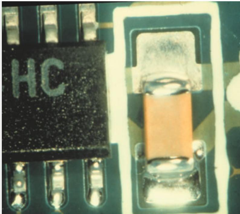
This specific problem can be overcome by altering the direction in which the board approaches the solder wave, but only if the layout engineer has foreseen the potential for this kind of defect and has made sure that there is at least one direction in which shadowing will not occur.
