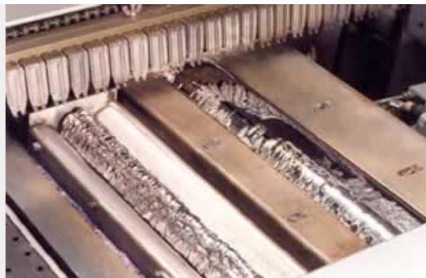
The primary or 'chip' wave is a symmetrical wave with an intentionally turbulent wave crest (Figure 3). The high kinetic energy at the point where the solder meets the board ensures that the solder finds its way to every joint on the board. A secondary wave then allows the solder to drain away from the board without leaving behind any bridges or unwanted accumulation of solder.
