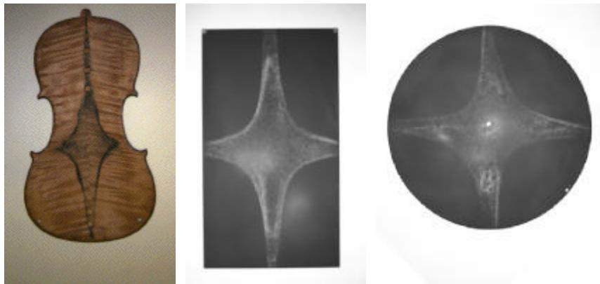
In this mode, opposite sectors of the plate are going up together, while adjacent sectors (separated by one node) are always moving in opposite directions. In the animation, the mode of the circular plate is shown, with the vertical motion both slowed and exaggerated to make it clear.
