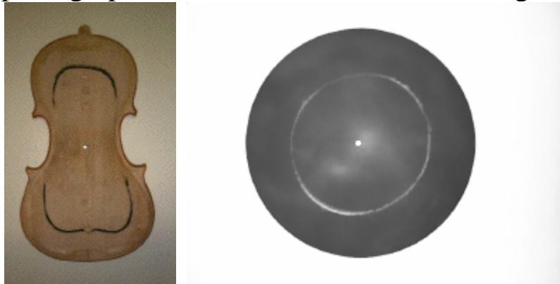
Mode 5 for the violin (called the ring mode) is comparable with the  $(0,1)$  mode of a circular plate. For a free plate, the centre of mass does not move, so when part of the plate moves up, another part moves down. In this mode, the central region moves in the opposite direction to the perimeter and only a ring remains motionless, as the animation shows.
