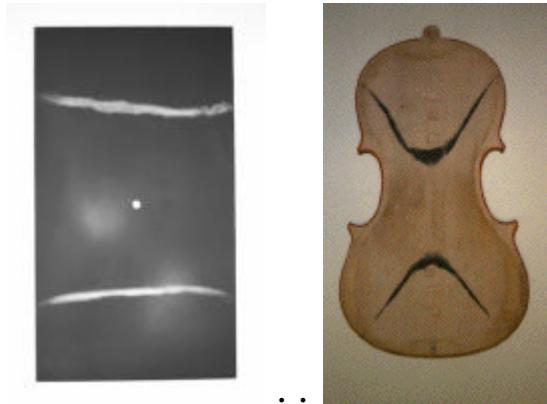
In these pictures, the lines are formed from sand that has collected at the nodes, but has been shaken off the moving regions. The violin back is more complicated in shape, and so the nodes also have a more complicated shape. White sand was used for the black-painted aluminium plate, and black sand for the violin back.
