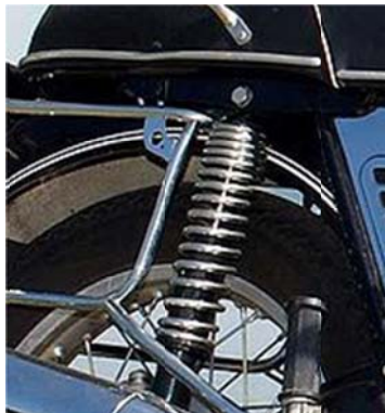
Fig. 7.19 Rear shock absorber and spring of a motorcycle
