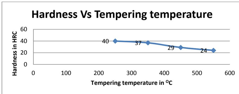
Figure: 7 Hardness Vs Tempering temperatures for tempering time of 90 min.
