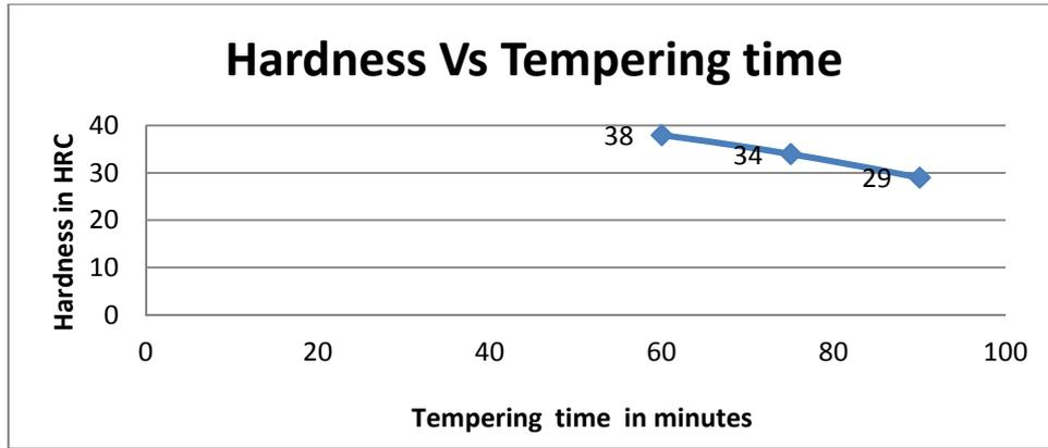
Figure: 3 Hardness Vs Tempering temperatures of 450°C
