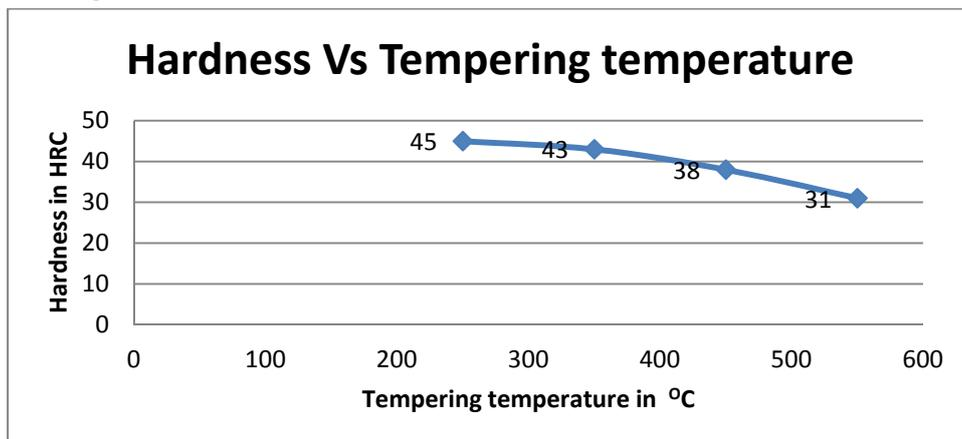
Figure: 5 Hardness Vs Tempering temperatures for tempering time of 60 min.
