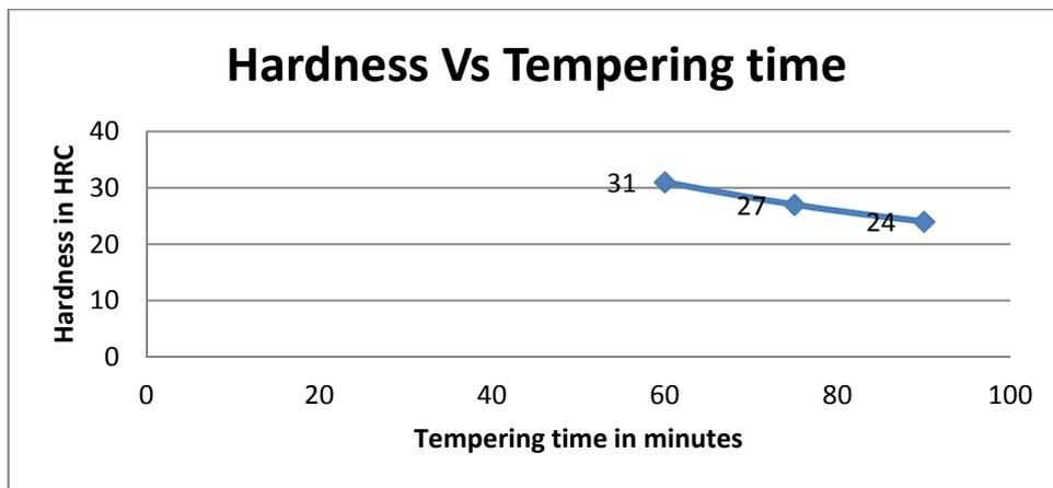
Figure: 4 Hardness Vs Tempering temperatures of 550°C
