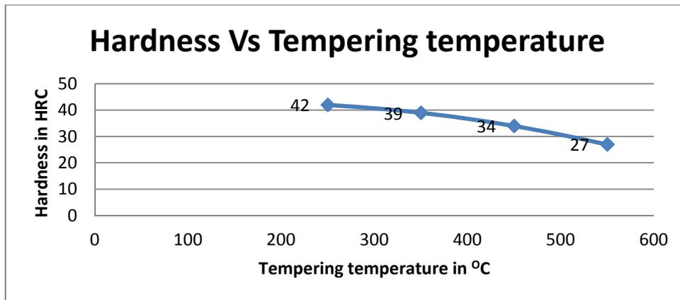
Figure: 6 Hardness Vs Tempering temperatures for tempering time of 75 min.
