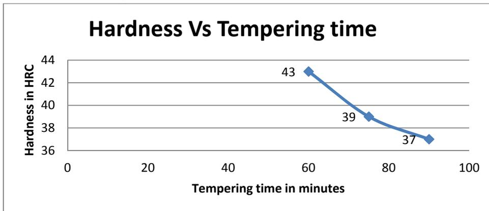
Figure: 2 Hardness Vs Tempering temperatures of 350°C
