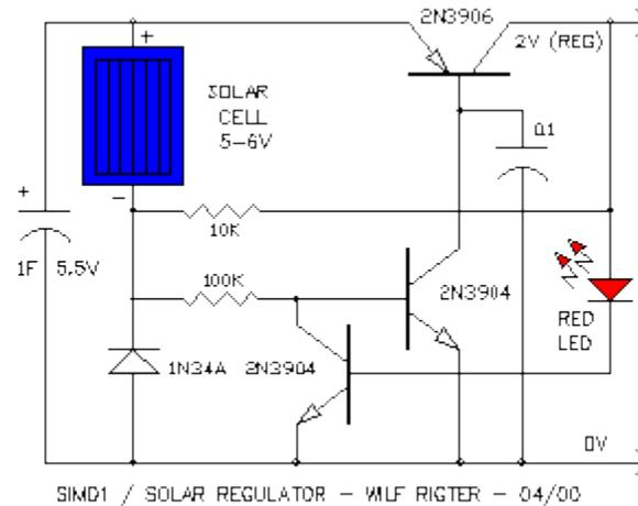
One interesting alternative would be to substitute a 5V NiCad (4 cell) battery for the 1F super cap which acts to increase the storage capacity many fold for use with flag waver motors, pendulums, etc. With higher load current, the 100K resistor may be replaced with 20K for up to 50 ma output current. The quiescent current of the regulator remains very low and is proportional to the load current for high efficiency operation during discharge.
