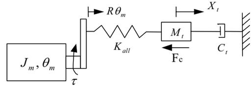
Fig. 6 Free-body diagram of the feed drive system.
