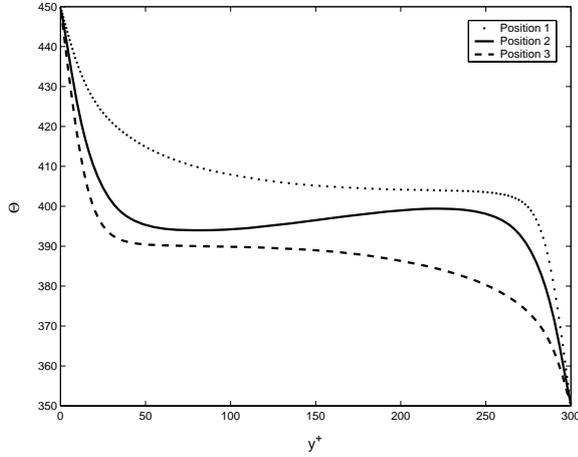
Fig. 3. Mean temperature profile at cross-stream positions 1, 2, and 3
