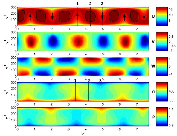
Fig. 1. Contour plot of stream-wise mean velocity  $U$ , wall-normal mean velocity  $V$ , cross-stream mean velocity  $W$ , mean temperature  $\Theta$ , and mean density  $\rho$ . The arrows on  $U$  contour plot show the direction of rotation of the Rayleigh-Benard counter-rotating vortices. The color bars to the right show the magnitude of the contours.
