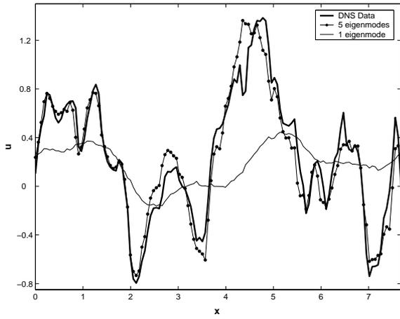
Fig. 7. Convergence of POD modes, contribution of 1 and 5 eigenmodes to  $u$ .
