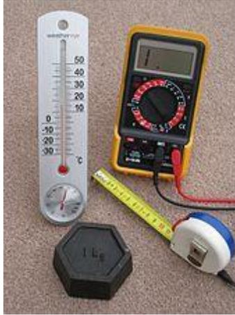
Four measuring devices having metric calibrations
