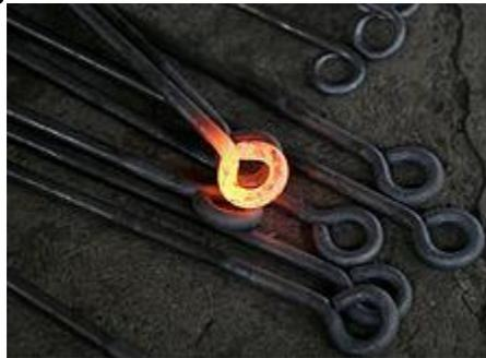
A red-hot iron rod from which heat transfer to the surrounding environment will be primarily through radiation.
