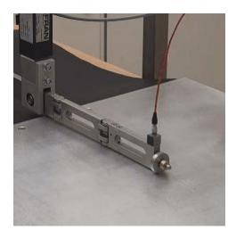
A physical model of the so-called 'Ziegler column', a two-degree-of-freedom system, exhibiting flutter instability as induced by dry friction. Watch the complete movie for more details.
