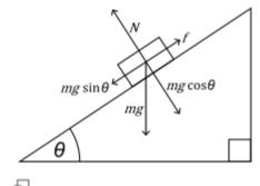
Angle of friction,  $\theta$ , when block just starts to slide.
