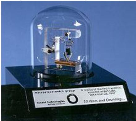
A replica of the first point-contact transistor in Bell labs
