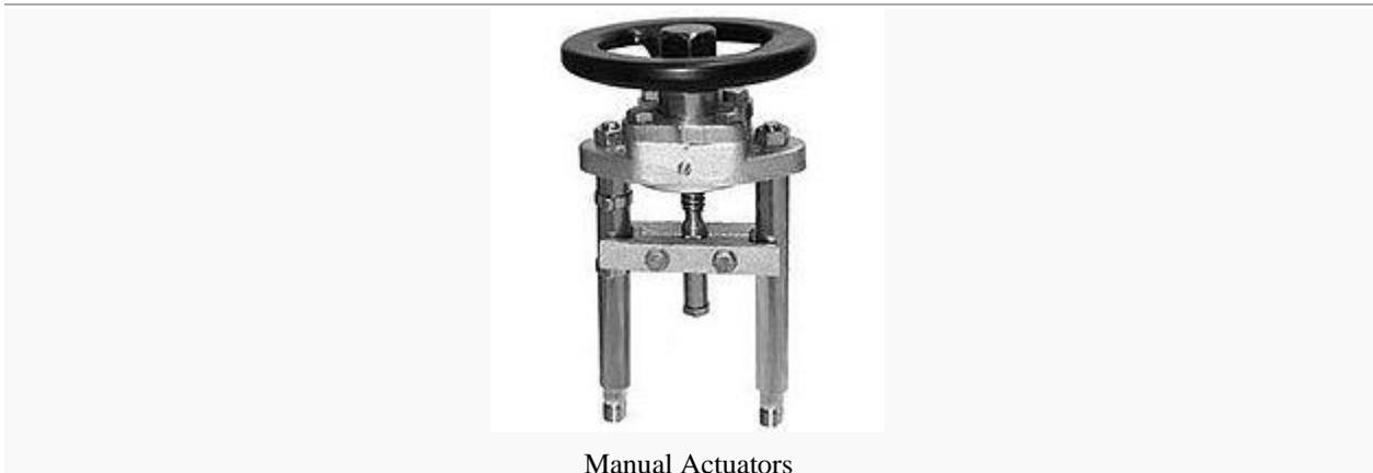
**Manual Actuators** are used in applications that require a throttling type of control valve that can be manually operated and set. Capable of giving precise manual throttling control, these actuators can be used on nearly all standard globe-style or angle-style valve body assemblies. A travel indicator on the actuator yoke can provide a visual indication of valve plug position.
