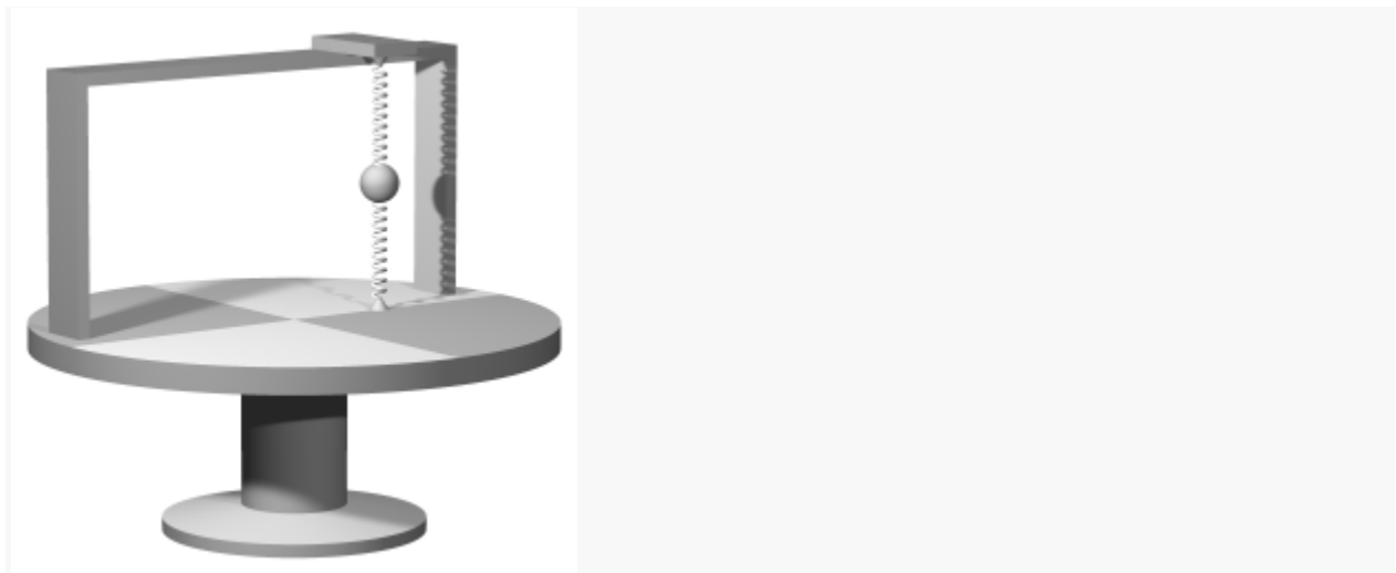
Picture 10. Image A Wheatstone pendulum setup with the attachment points aligned with the central axis of rotation.
