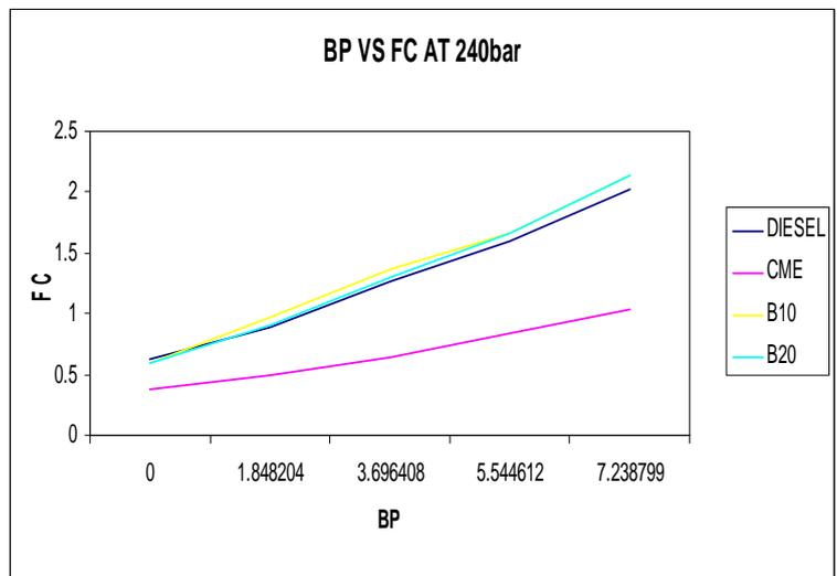
**FC of diesel, biodiesel and its blends at 240 bar injection pressure**
