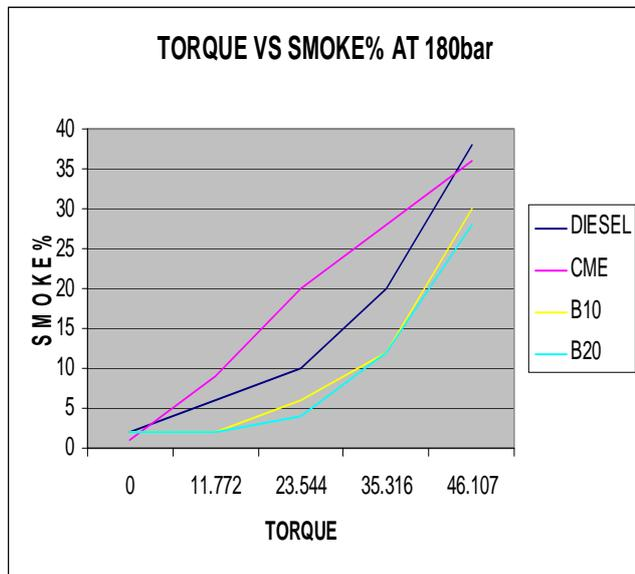
**Smoke density of diesel and biodiesel and its blends at 180 bar injection**
