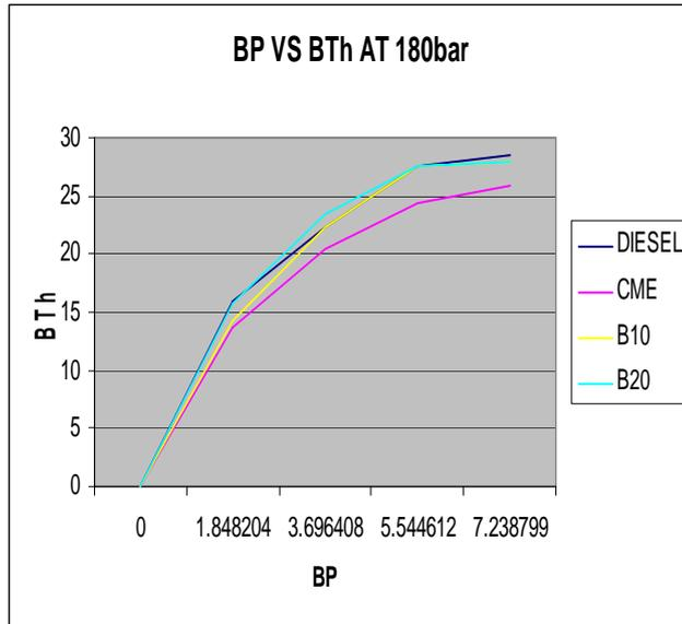
**Brake thermal efficiency of diesel, biodiesel and its blends at 180 bar injection pressure**
