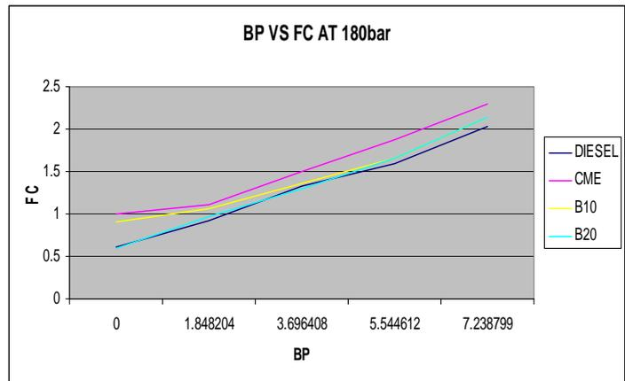
**FC of diesel, biodiesel and its blends at 180 bar injection pressure**
