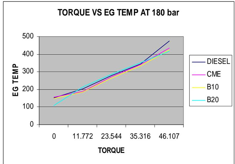
**Exhaust temperatures of diesel biodiesel and its blends at 180 bar injection pressure**
