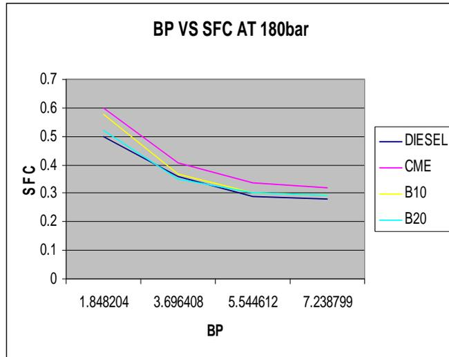
**SFC of diesel, biodiesel and its blends at 180 bar injection pressure**
