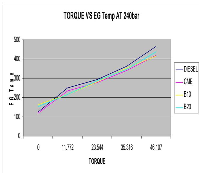
**Exhaust temperatures of diesel biodiesel and its blends at 240 bar injection pressure**
