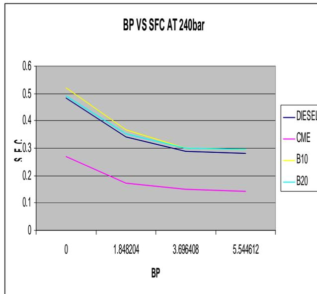
**SFC of diesel, biodiesel and its blends at 240 bar injection pressure**
