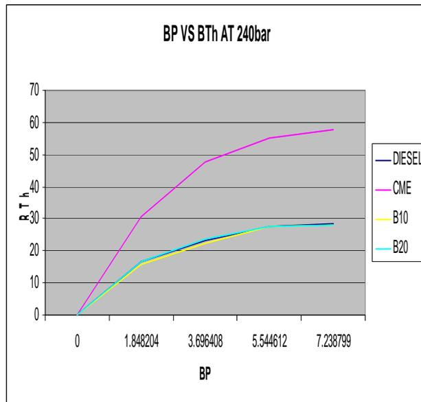
**Brake thermal efficiency of diesel, biodiesel and its blends at 240 bar injection pressure**
