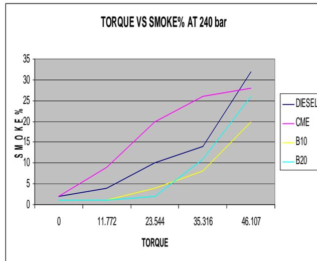
**Smoke density of diesel and biodiesel and its blends at 240 bar injection**
