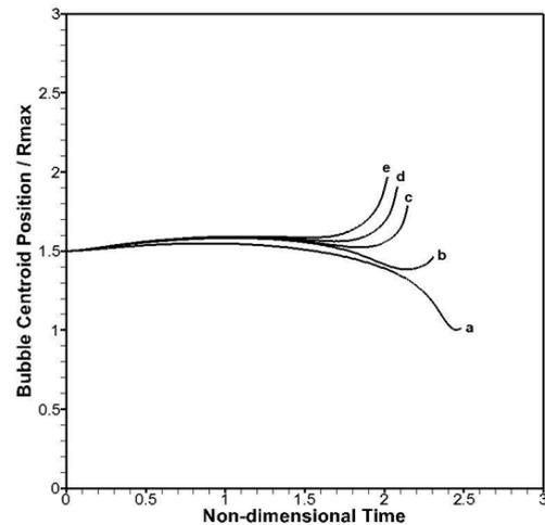
Fig. 9. Movement of the bubble centroid with respect to non-dimensional time during its growth and collapse phases near a rigid boundary and near a thin bronze plate with different thicknesses. (a) Rigid boundary, (b)  $th^* = 0.0089$ , (c)  $th^* = 0.0086$ , (d)  $th^* = 0.0083$  and (e)  $th^* = 0.008$ . The bubble is characterized by  $\gamma = 1.5$ ,  $\delta = 0$  and  $\varepsilon = 10$ .
