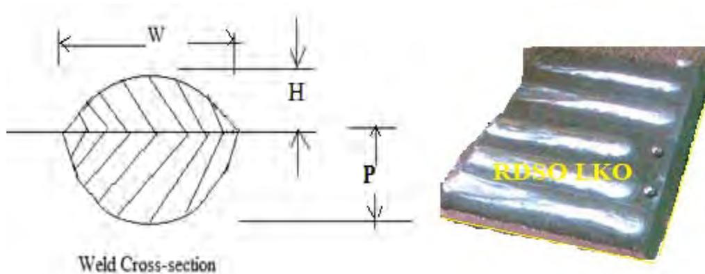
Fig.2 Weld bead Penetration (P)
