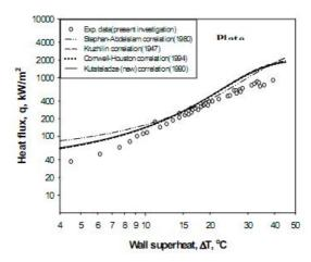
Figure 3 Comparison of pool boiling experimental result of water with existing correlations
