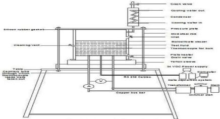
Figure 1 plae heater pool boiling experimental setup
