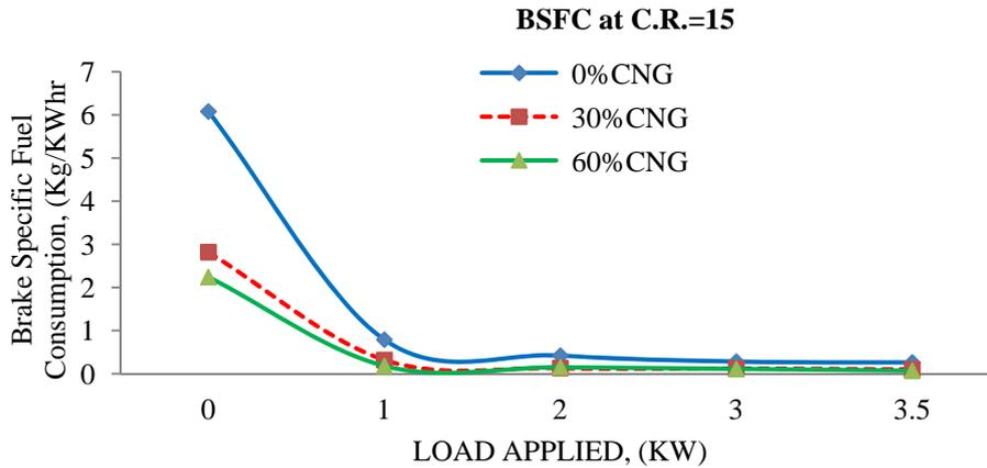
Fig. 5.:Brake specific fuel consumption with load for diesel and dual fuel mode at C.R.=15
