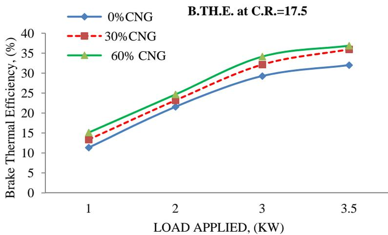
Fig.4: Brake thermal efficiency with engine load for pure diesel and dual fuel mode at C.R. =17.5.
