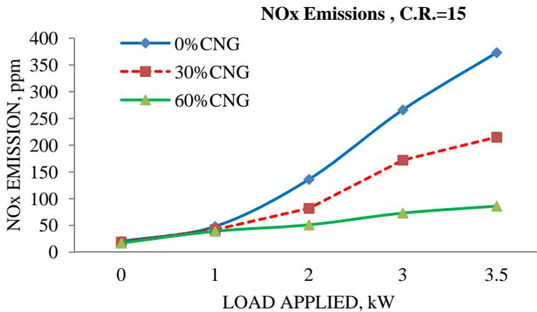
Fig.13:  $\text{NO}_x$  Emission as a function of engine load for diesel and dual fuel modes at C.R. =15.
