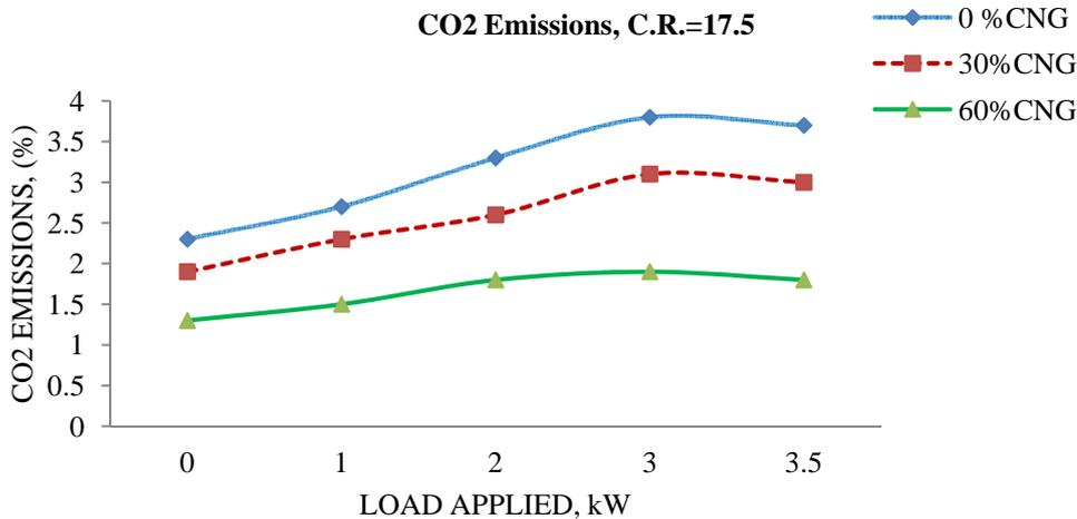
Fig.12: CO<sub>2</sub> Emissions for diesel and dual fuel mode of operation at C.R. =17.5.
