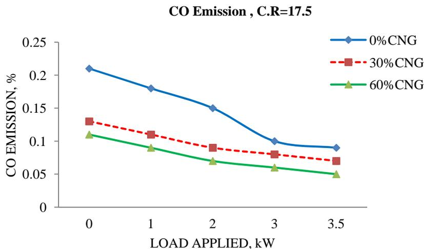
Fig.8: CO Emission with load applied for pure diesel and dual fuel modes at C.R=17.5.
