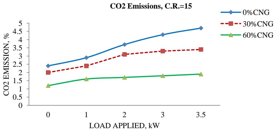
Fig. 11: CO<sub>2</sub> Emissions for diesel and dual fuel mode of operation at C.R. =15.
