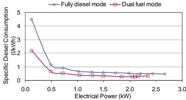
Fig. 4. Specific Diesel Consumption at various electrical loads
