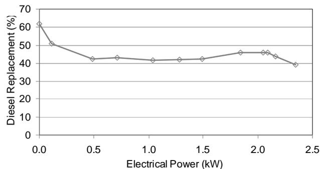
Fig. 3. Diesel Replacement Percentage in dual fuel mode
