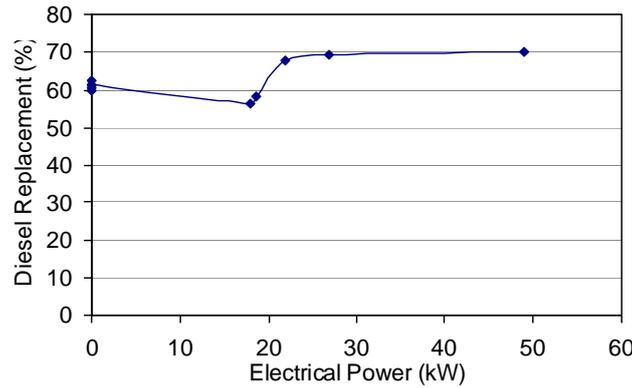
Fig. 7. Diesel Replacement Percentage in dual fuel mode for 100 kW DG set
