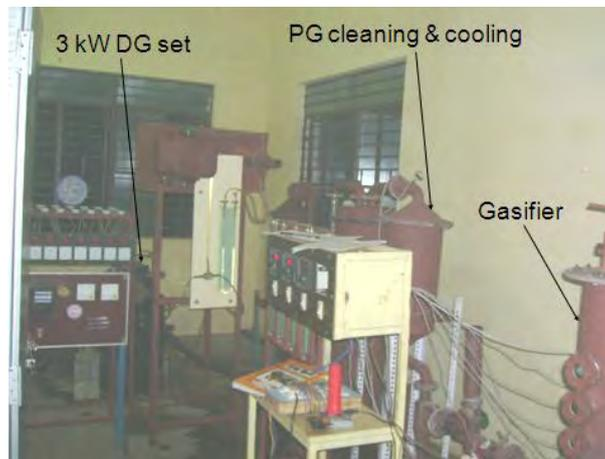
Fig. 1. Experimental gasifier-engine-generator system
