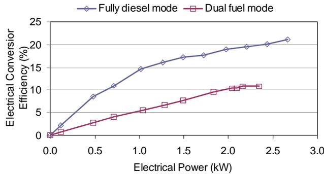
Fig. 5. Electrical Conversion Efficiency at various electrical loads
