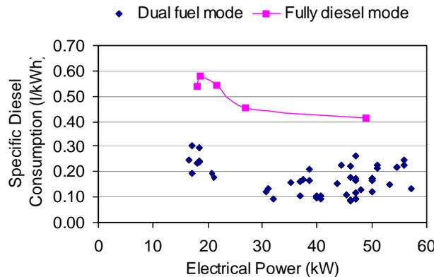
Fig. 8. SDC of 100 kW DG set at various electrical loads
