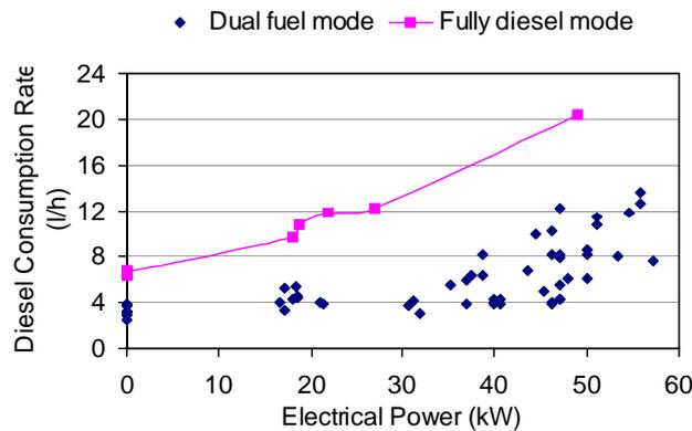
Fig. 6. DCR of 100 kW DG set at various electrical loads
