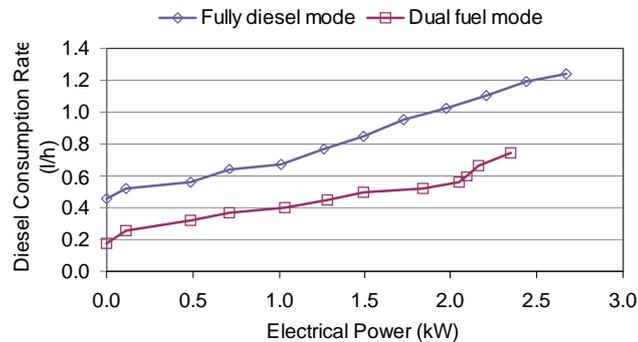
Fig. 2. Diesel Consumption Rates at various electrical loads
