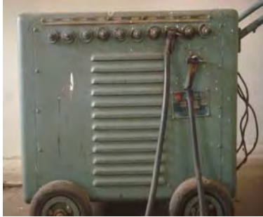
Fig. 1 Johnson arc welding transformer
