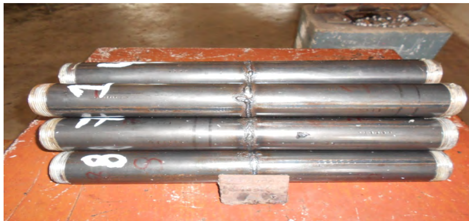
Fig. 4 Welded tubes with threaded ends wound with Teflon
