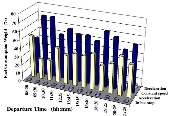
Fig. 11 Distribution of fuel consumed to characteristic processes for MODE 1 and MODE 2
