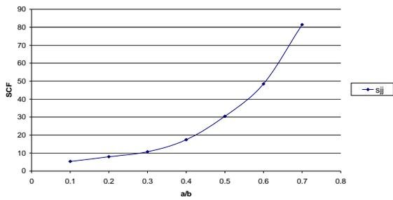
Fig. 9 SCF Vs a/b ratios of single-J butt welded joint
