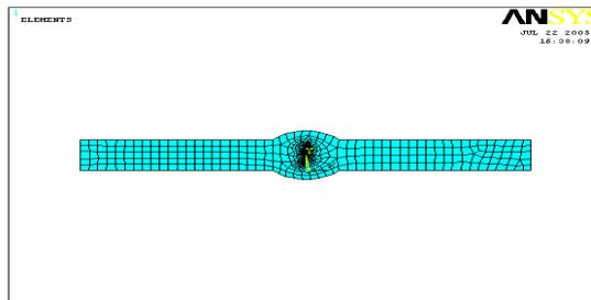
Fig. 2 Meshed model of a Double-V butt-welded joint
