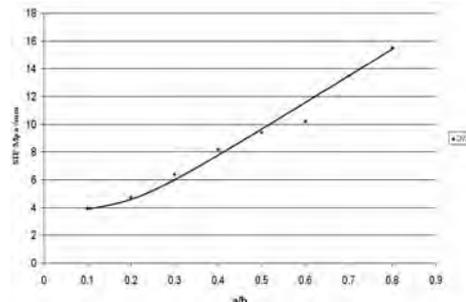
Fig.4 SIF Vs a/b ratios of double v butt-welded joint
