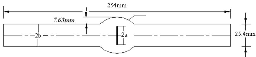
Fig. 1 Geometric model of the tested specimen
