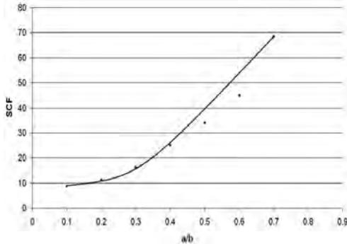
Fig. 5 SCF Vs a/b ratios of single-V butt-welded joint
