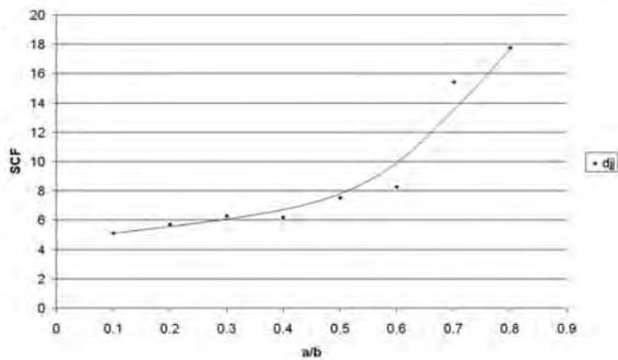
Fig. 7 SCF Vs a/b ratios of double J butt-welded joints
