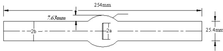
Fig. 1 Geometric model of the tested specimen
