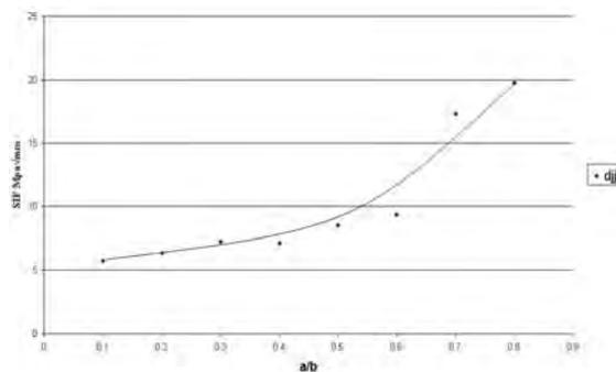
Fig.8 SIF Vs a/b ratios of double J butt-welded joint
