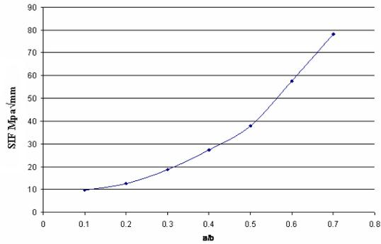
Fig. 6 SIF Vs a/b ratios of single-V butt-welded joint.
