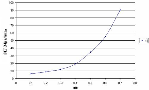
Fig. 10 SIF Vs a/b ratios of single J butt-welded joint
