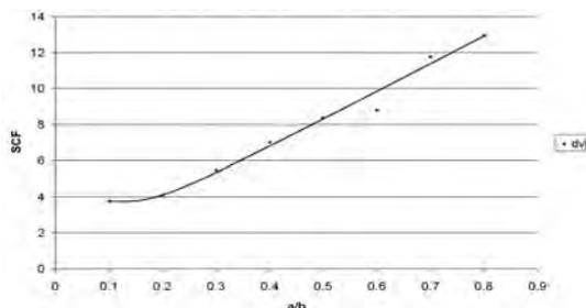
Fig. 3 SCF Vs a/b ratios of double V butt-welded joint
