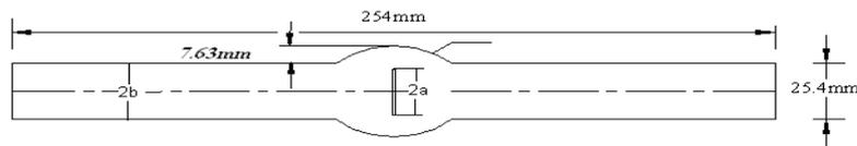
Fig. 1 Geometric model of the tested specimen
