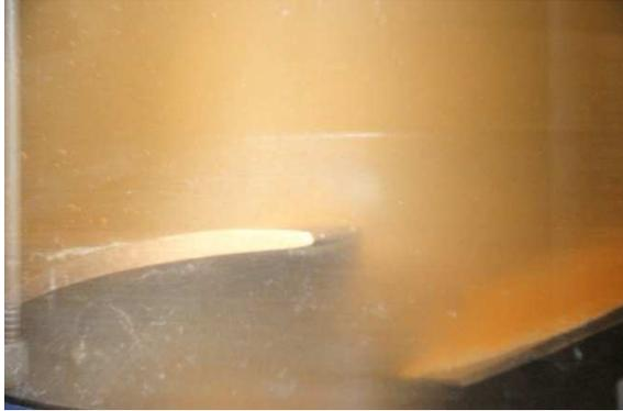
Fig. 1 Cavitation pattern under operating condition of No. 1-1
