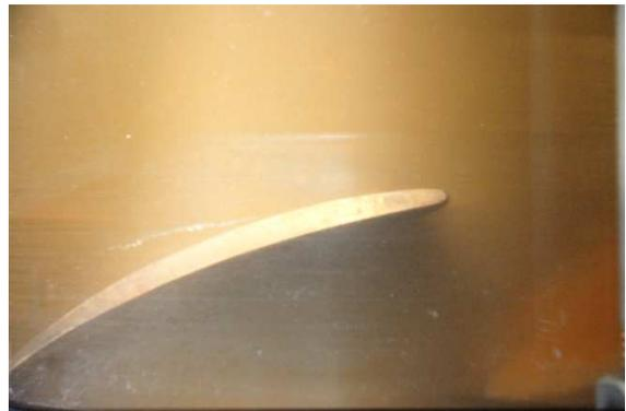
Fig. 6 Cavitation pattern under operating condition of No. 2-1
