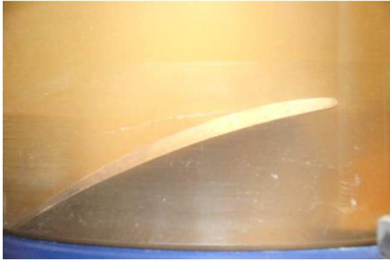
Fig. 7 Cavitation pattern under operating condition of No. 2-2
