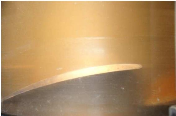
Fig. 3 Cavitation pattern under operating condition of No. 1-3
