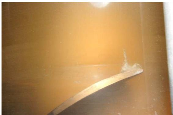
Fig. 13 Cavitation pattern under operating condition of No. 3-3
