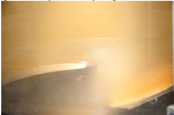
Fig. 4 Cavitation pattern under operating condition of No. 1-4
