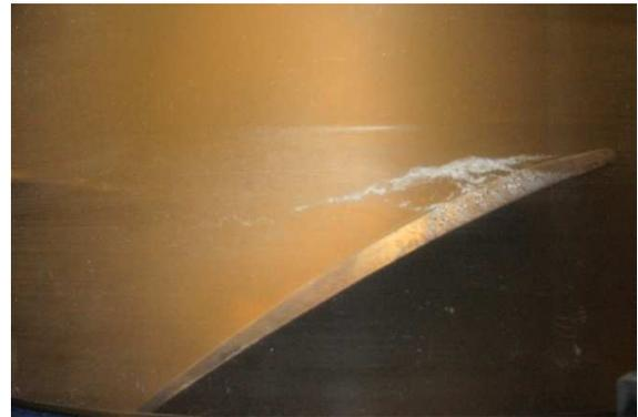
Fig. 12 Cavitation pattern under operating condition of No. 3-2
