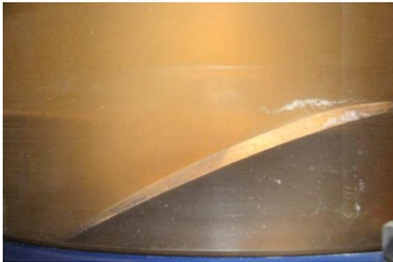
Fig. 8 Cavitation pattern under operating condition of No. 2-3
