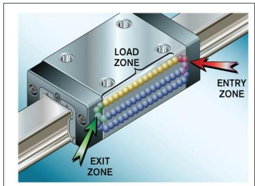
True high-precision performance with linear guides is only possible by limiting unwanted motion in the X, Y, and Z axes as the runner block travels along the rail; this can be done by optimizing ball recirculation inside the runner block.
