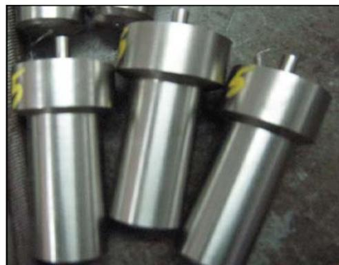
Fig. 2 Fabricated FSW tools
