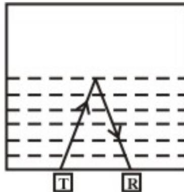
Fig. 3 Level measurement using ultrasonic technique
