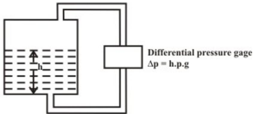
Fig. 1 Level measurement using hydrostatic differential pressure
