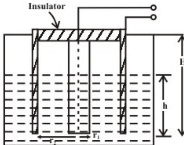
Fig. 2 Level measurement using capacitance technique
