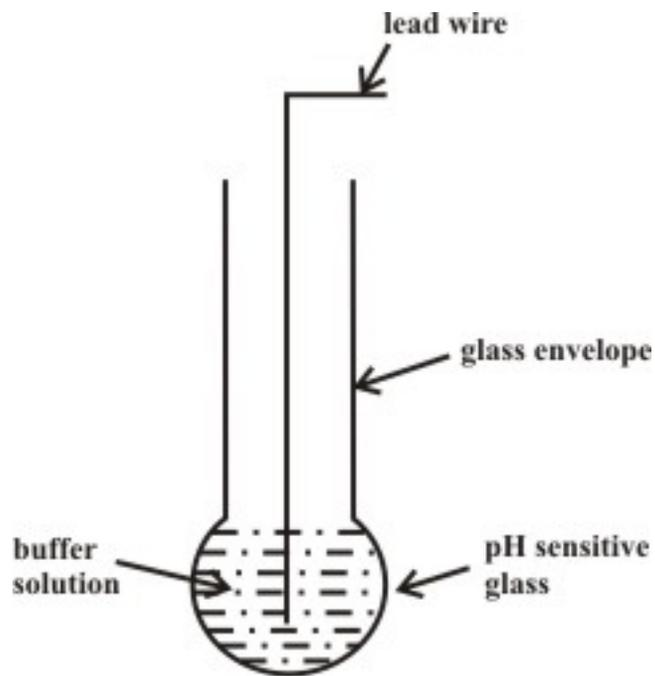
Fig. 7 Measuring Electrode
