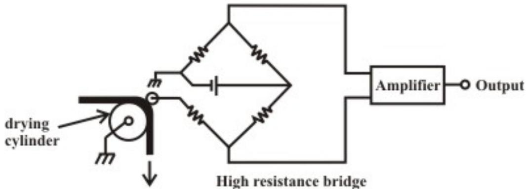
Fig. 6 Moisture measurement using resistive technique
