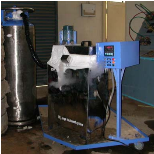
Fig.1. The Cryogenic Treatment Chamber
