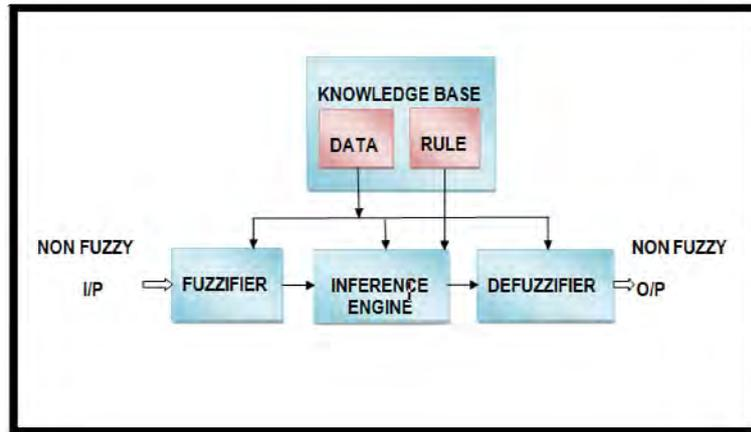
Fig.1.The structure of fuzzy expert systems
